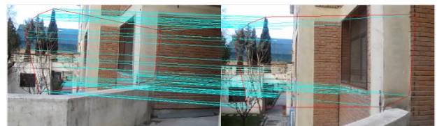
Figure 1. Inseparation of far from close obstacles in Al-Kaff et al's algorithm
