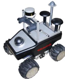
Figure 4: UGV Summit XL (Robotnik) carrying LiDAR and stereo camera
