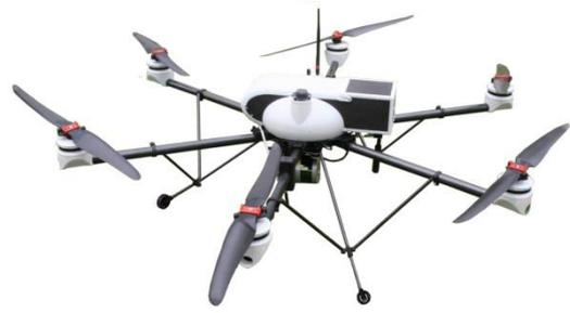
Figure 2: UAV Typ “AR200” carrying a LiDAR
