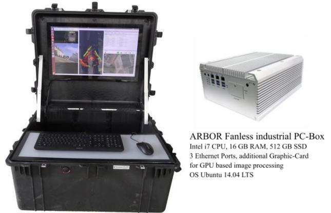
Figure 7: Ground-Station-PCBox (ARBOR FPC-7800-Series)
