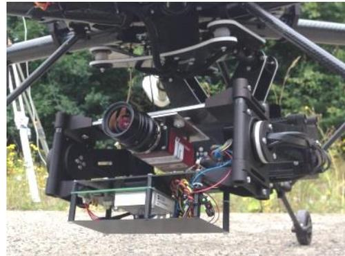
Figure 3: 2-axis-gimbal carrying a RGB-camera
