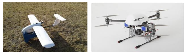
Figure 3. The Skywalker fixed-wing UAV and the AKS Raven X8 multi-rotor UAV.
