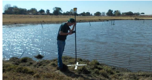
Figure 1. Placement of the ground control markers.
