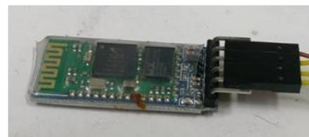
Figure 3 HC-05 wireless blue tooth module
