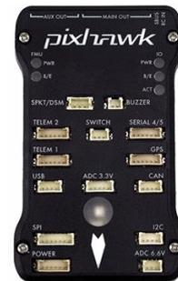
Figure 1 Pixhawk flight control board
