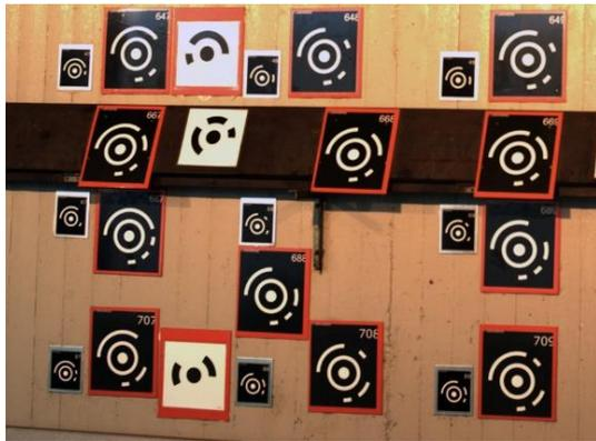
Figure 1b. Different types of coded targets
