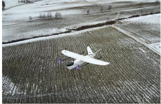
Figure 2. Hybrid UAV with enhanced rotary-wing capabilities, hovering 50 m AGL over the test location at Apelsvoll research station (image taken from a multi-rotor UAV)
