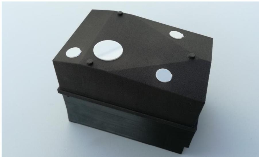
Figure 1. Photo of the *FGI Aerial Image Reference System*. The three small cosine collector optics belonging for the RGB photodiodes are all tilted 10° to opposite directions.
