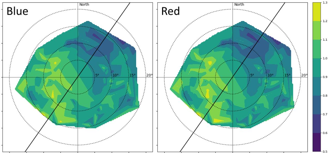
Figure 2. Reading of a single irradiance sensor vs its tilt as measured in a ground based experiment. During the measurement sky was mostly blue with thin cirrus clouds in front of the sun. Solar zenith angle was approximately  $42^\circ$ . The thick line across the plot indicates the solar principal plane. The intensity units are relative to horizontal measurement.
